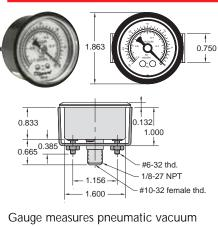
Gauge measures pneumatic vacuum pressure. Mounting bracket included.
